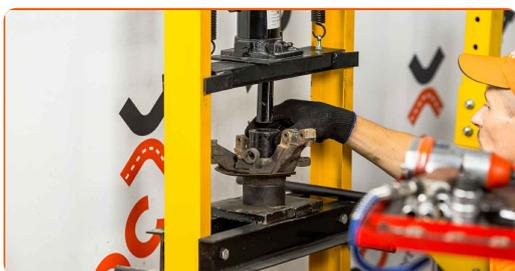
Înlocuirea: rulment roata – VAUXHALL Corsa Mk II (C) Hatchback (X01).
